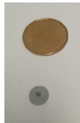
Distance ring for motor slide valve
